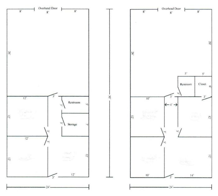
The above drawings are typical of what an office/warehouse will look like. Both of the drawings are 1,200 square feet. The office/warehouse will be a minimum of 1,000 square feet and a maximum of 1,400 square feet.
